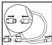
1. Connect the PREVENA™ Therapy V.A.C.® Connector to the PREVENA PLUS™ Connector:
