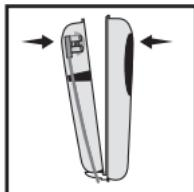
1. Ensure canister is securely locked onto the therapy unit. When canister is installed, a distinct click will be heard indicating it has been properly installed.
