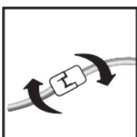
3. Check tubing connectors to ensure they are fully engaged and locked.
