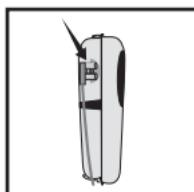
2. Check dressing tubing connector at canister.
